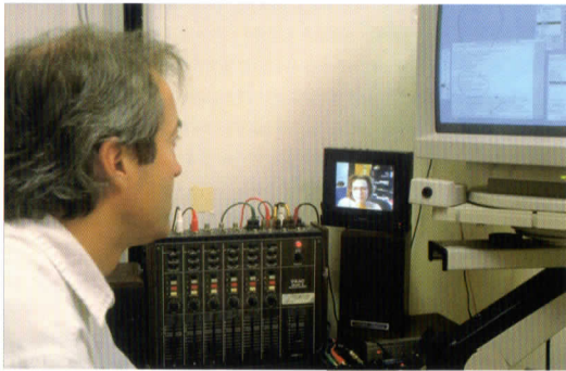
Figure 1 ◀ A Typical Desktop Video Conferencing Configuration. Conferencing is typically channeled through a video camera on top of a monitor on the user's desktop.
