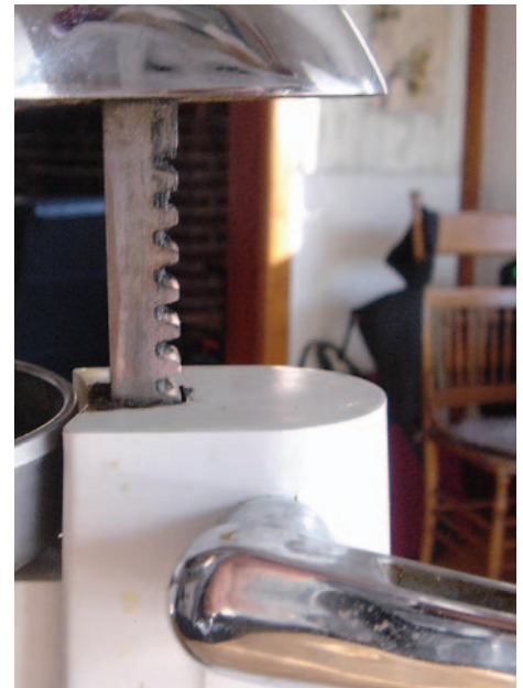
Figure 4: Gear Mechanism of the Mighty OJ Rotary motion of the arm raises and lowers the “jaws” of the juicer by means of a rack and pinion gear. The gear ratio is constant.
