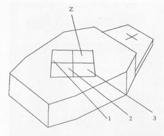
this paper, they shall be referred to as the *Z-button*, and *buttons* 1–3. When the tracker is placed in a particular position different events can be generated depending on which button is depressed. This is a useful interaction that cannot be realized using, for example, a stylus or lightpen, without using a second hand.
