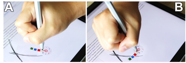
Figure 5. The Palm Tools rotate to match the “up” direction in the hand-centric reference frame of the sensed palm.
