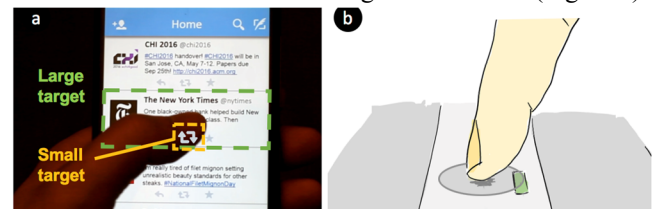
Figure 10. Twitter mockup. (a) Each tweet (large target) contains reply, retweet, and favorite icons (small targets). (b) Precise pointing redirects to a nearby small target.
